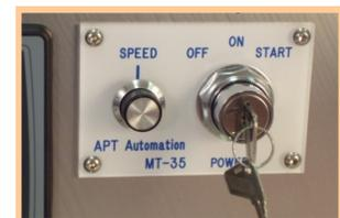
Safety power lockout via key switch when power resumes after power loss or operator shut down.
