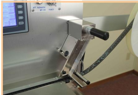
Optional de-tape module removes old cover tape from a finished reel and simultaneously applies a new cover tape without a reduction in throughput.
