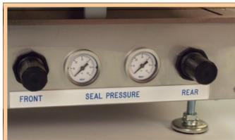
Independent pressure and temperature control for each seal shoe for excellent front to back seal symmetry.
