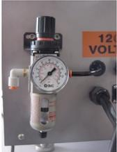
Incoming air pressure regulation is built-in along with low pressure sensing and alarming to avoid production loss due to pressure-related seal problems.
