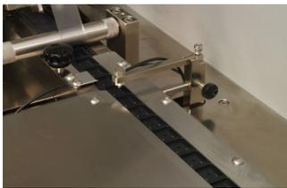
Reliable missing parts detection via optical sensing guarantees that every pocket in a production run is full. (OPTIONAL)
