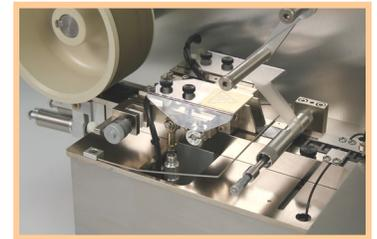
Advanced multi-mode sealing station seals thermal or PSA tapes.
